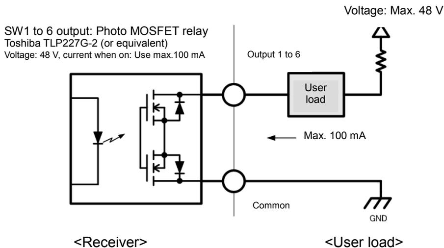
The receiver uses photo MOSFET output. When a load is connected, use a voltage of 48 V or less with a current of 100 mA or less during output.
