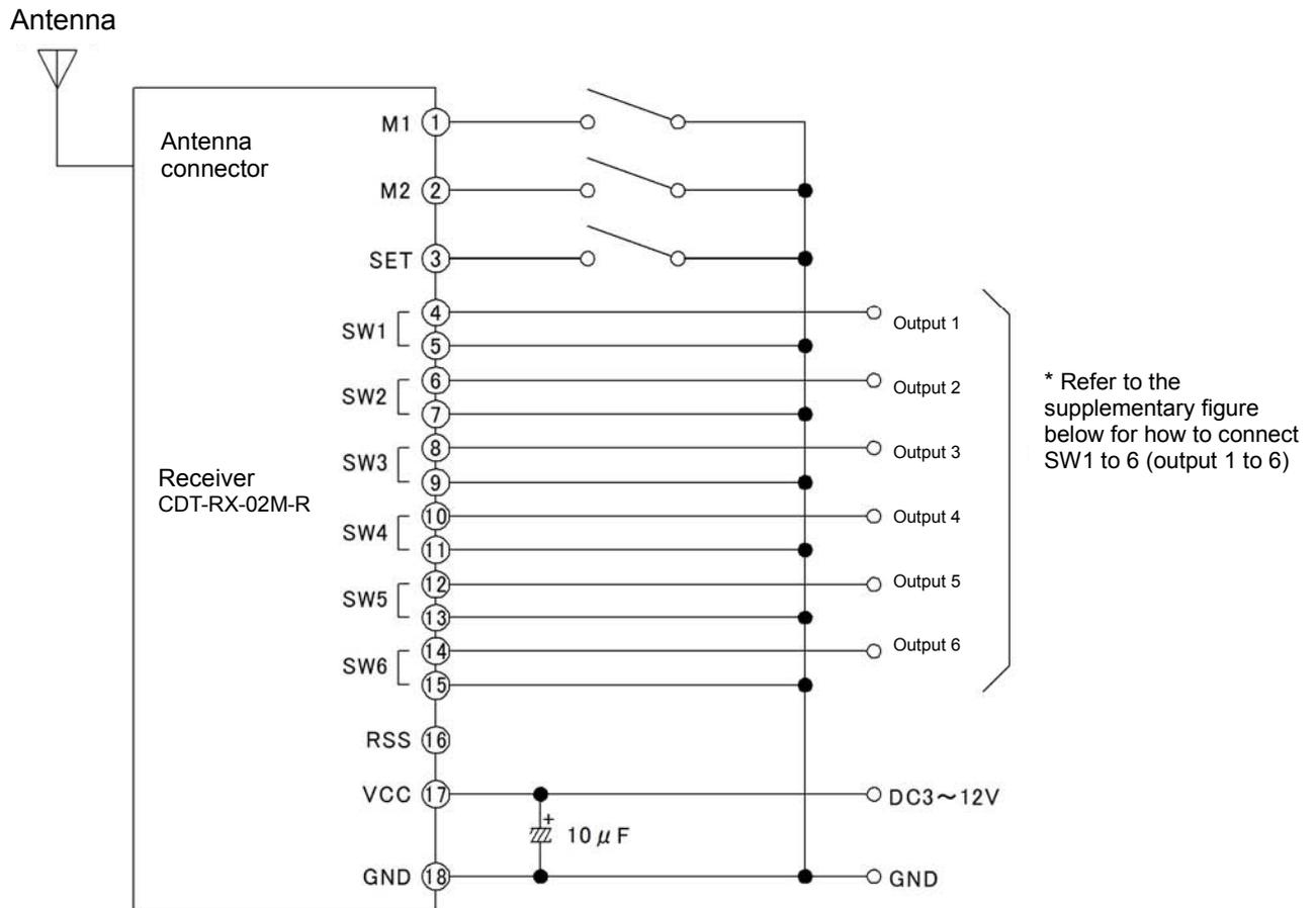
**\* Supplementary figure: SW1 to SW6 (Output 1 - 6) connection**
