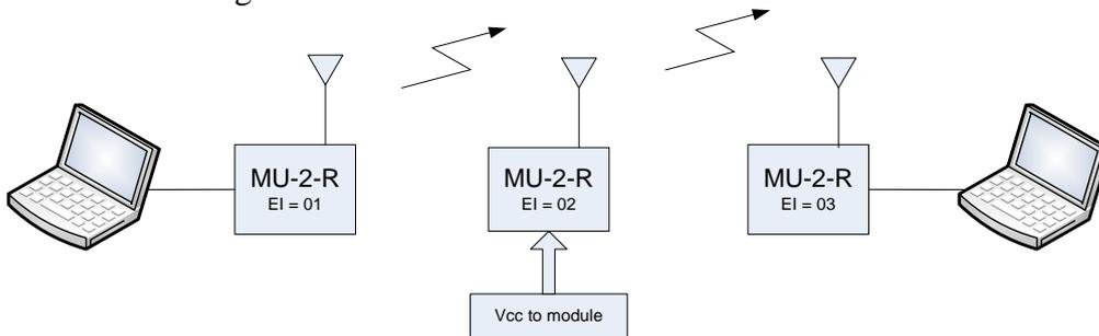
The relay module will require only Vcc and GND to function. You can:
