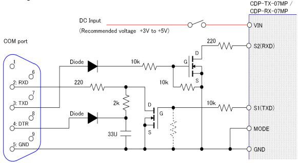
For the FETs, general switching FETs (N-ch) operating at low voltage can be used. Transistors (NPN) are also usable.
