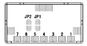
The solder jumpers JP1 and JP2 are internally connected to the pin  $\,$  # 6 and pin #7, respectively.
