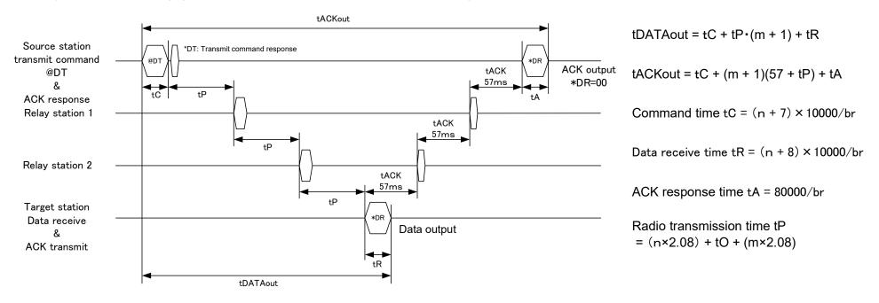
\* Units are ms, n=Number of data bytes sent(within 255 bytes), br=UART bit rate, M=Number of relays (up to 10 units), t0=Overhead Table 2 \* Reference value 1 with 20-byte link data: tDATAout=262 ms, tACKout=429 ms Conditions: Standard mode, 57,600 bps, 2 relays \* Data output time when there is no ACK response is calculated with tDATAout
