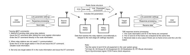
When using the MU-4 to transmit data, it is first necessary to perform various initial settings. When an MU-4 setting command is issued, a command response corresponding to the command is always returned from the MU-4. Process the command response as necessary. In addition, when data is received from the source station, a data receive is output from the target station, so perform receiving process according to its data size.
