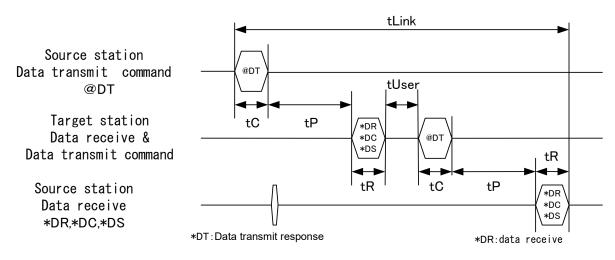
Command time  $tC = (n+7) \times 10000 / br$ Radio transmission time  $tP = (n \times 2.08) + tO$ Data receive time  $tR = (n+8) \times 10000 / br$ tUser = User program processing timetLink = Time to establish link\*Units are ms\*n = number of data bytes sent (within 255 bytes)\*bR = UART bit rate\*tO = Overhead Table 1\*Reference value with 20-byte link data.\*ink data.\*ink data
