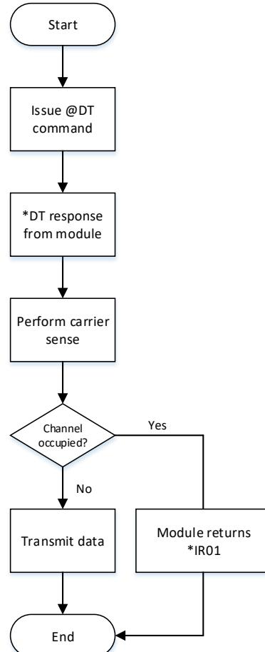
3. SLR-434M and SLR-429M LoRa® modulation. Both carrier and correlation sensing performed.
